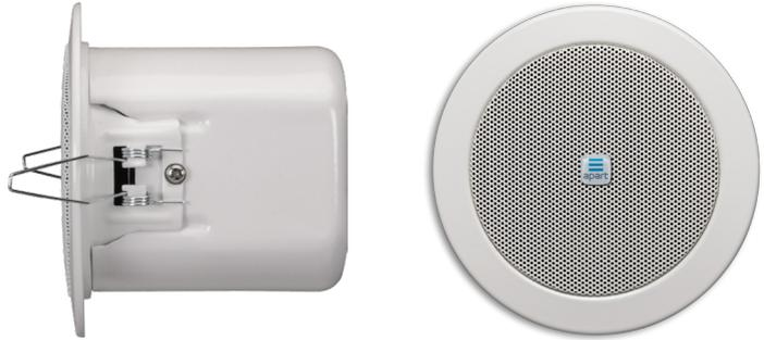
The CM4 is a stylish small built-in low impedance loudspeaker. Thanks to its halogen-spot size, it can be integrated into any interior style. It is ideal for speech and backgroundmusic in quiet areas, toilets, cloakrooms, ... The speaker has a full metal frame, a metal back can and a coated dual paper cone for the lowest distortion and increased resistance against moisture. The CM4 is easy to install thanks to its simple, quick mounting system (2 spring clamps).
