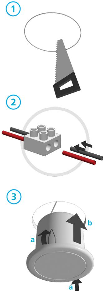
**The loudspeaker is easy to install, due to its simple mounting system.**
