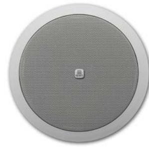
The CM20T two-way built-in loudspeaker can be used as a 16 ohms or 100 volt loudspeaker. In 16 ohms use, you can connect up to 4 loudspeakers in parallel on each channel of a standard 4 ohms amplifier. For 100 volt use, the CM20T is equipped with a high-quality 20 watts 100 volt transformer with several power tapings (20 – 10 – 5 – 2.5 watts). Therefore it can be used in projects with high ceilings or places with background noise where a little more power is needed.
