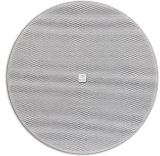
The Apart CM20DT is a 2-way 100V / 70V / 16 ohm built-in design ceiling loudspeaker. The loudspeaker has a 6 ½" woofer, a 1" coaxial tweeter and a high quality 100 / 70 volt loudspeaker line transformer with multiple power taps. CM20DT is the perfect choice for the distribution of microphone calls and background music. The mounting frame is made of high quality ABS. The steel grille is kept in place by strong magnets.
