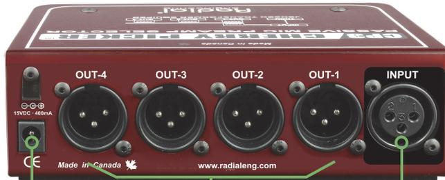
**POWER & CABLE CLAMP** for the included 15VDC power supply. Clamp prevents disconnection.
