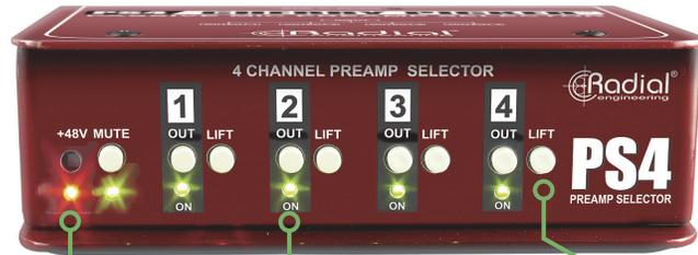
**BUILT IN 48V - PHANTOM** for condenser mics and active DI's. Switch is recessed to prevent accidental turn-on.
