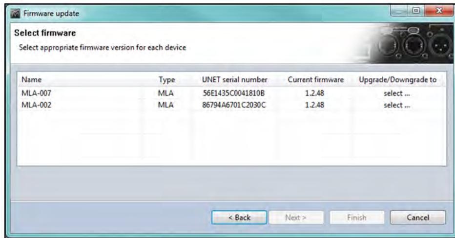
The current firmware is shown and the final column has an option to select the required firmware which in most cases would be a new version but could be an old firmware if say a bug has been found in a current version and it is necessary to downgrade to an earlier version. If there are several versions available, clicking on the Upgrade/Downgrade cell will bring up a drop-down showing the version numbers. Select the version you wish to use and it will appear in the final column; -
