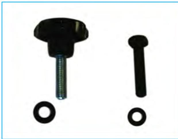
The handwheel is for portable applications where adjustment is necessary once the speaker is in position, the M8 x 40mm bolt is for permanent installations where the tilt adjustment needs to be tightened off permanently.
