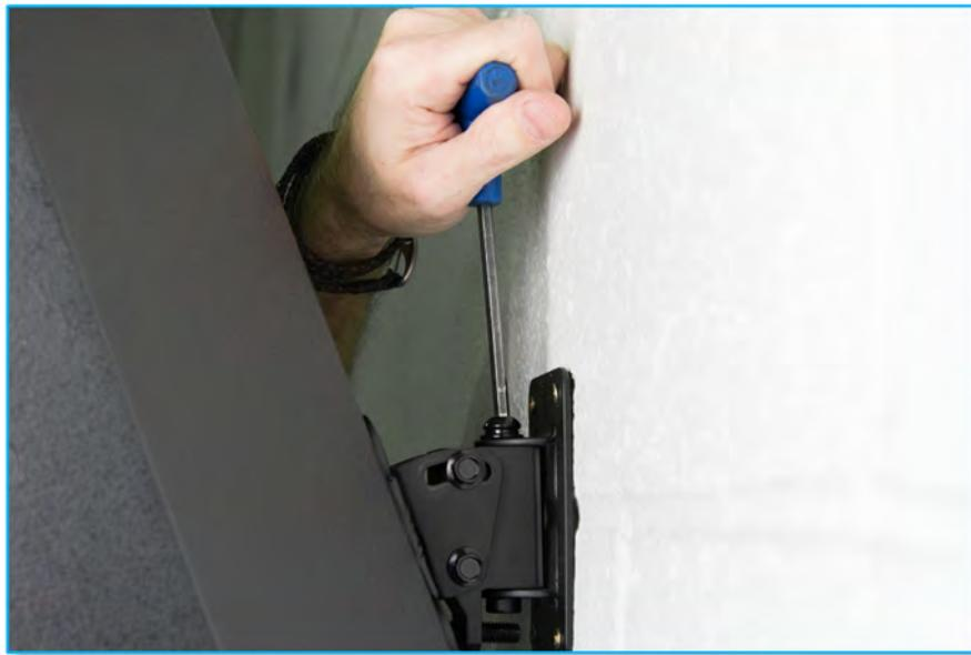
Vertical (tilt) adjustment is made by adjusting the grub screw:
