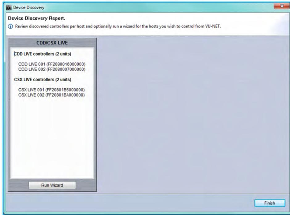
There are no array configuration options so clicking on 'Run Wizard' simply synchronises the cabinets with Vu-Net so that what is displayed in the application is exactly the configuration of the connected cabinets; -
