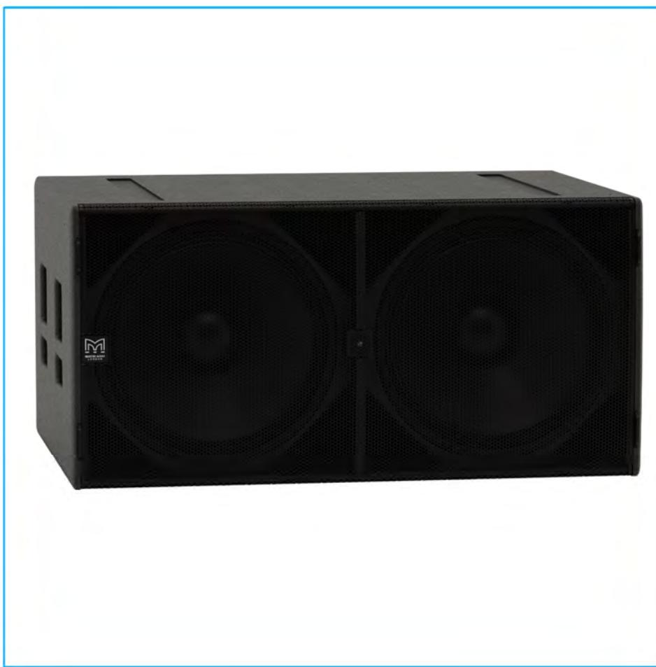
The SXP218 achieves the ultimate in subwoofer performance for the most demanding professional applications – delivering very high output levels and superb transient performance with minimal distortion. With an operating range of 35Hz- 150Hz ± 3dB, it houses dual 18" long-excursion (460mm)/4" (100mm) voice coil drivers with water-resistant cones and triple roll surrounds.
