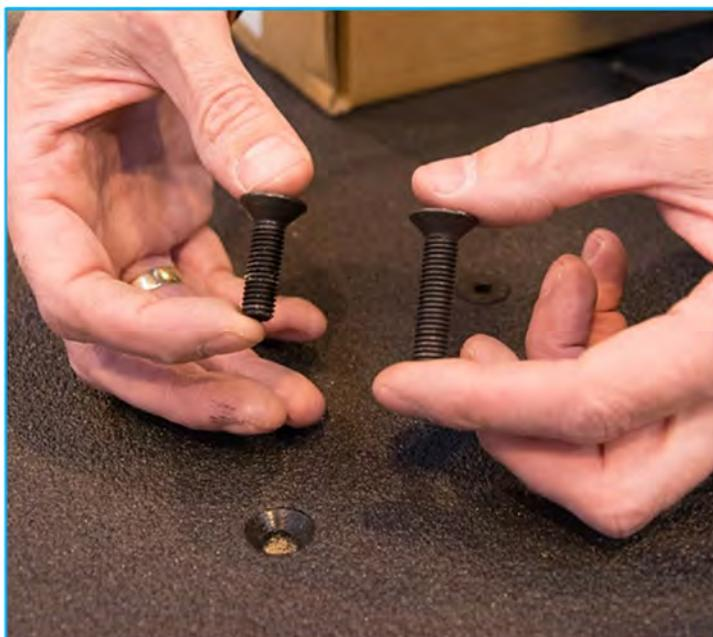
Position the bracket and attach with the M8x35mm screws and fully tighten;
