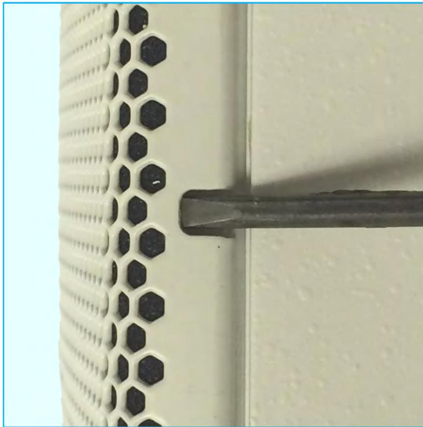
Push the handle down a little first. This will ease the grille out of the slot.
