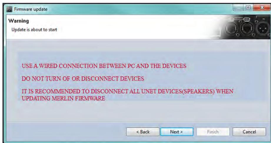
Click 'Next' and the upgrade will start. A progress window will appear showing the processes in the upgrade taking place. The system tackles one device at a time, placing it into Boot Mode, uploading the firmware and rebooting the device back into an operating mode; -
