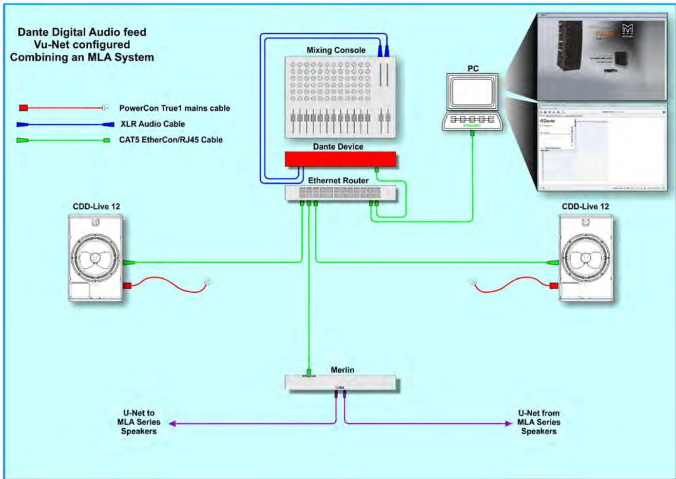
CDD-Live is ideally suited to being integrated with a Martin Audio Multicellular system, the entire system can be managed via a single Vu-Net project.
