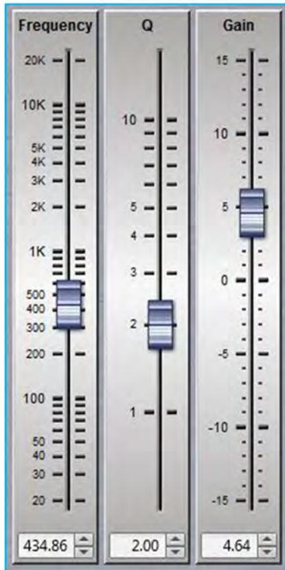
Parameters can be changed on the properties panel in three ways. The faders can be drag and dropped to a new value, the value can be scrolled up or down using the up/down buttons to the right of the value windows, and finally values can be directly typed
