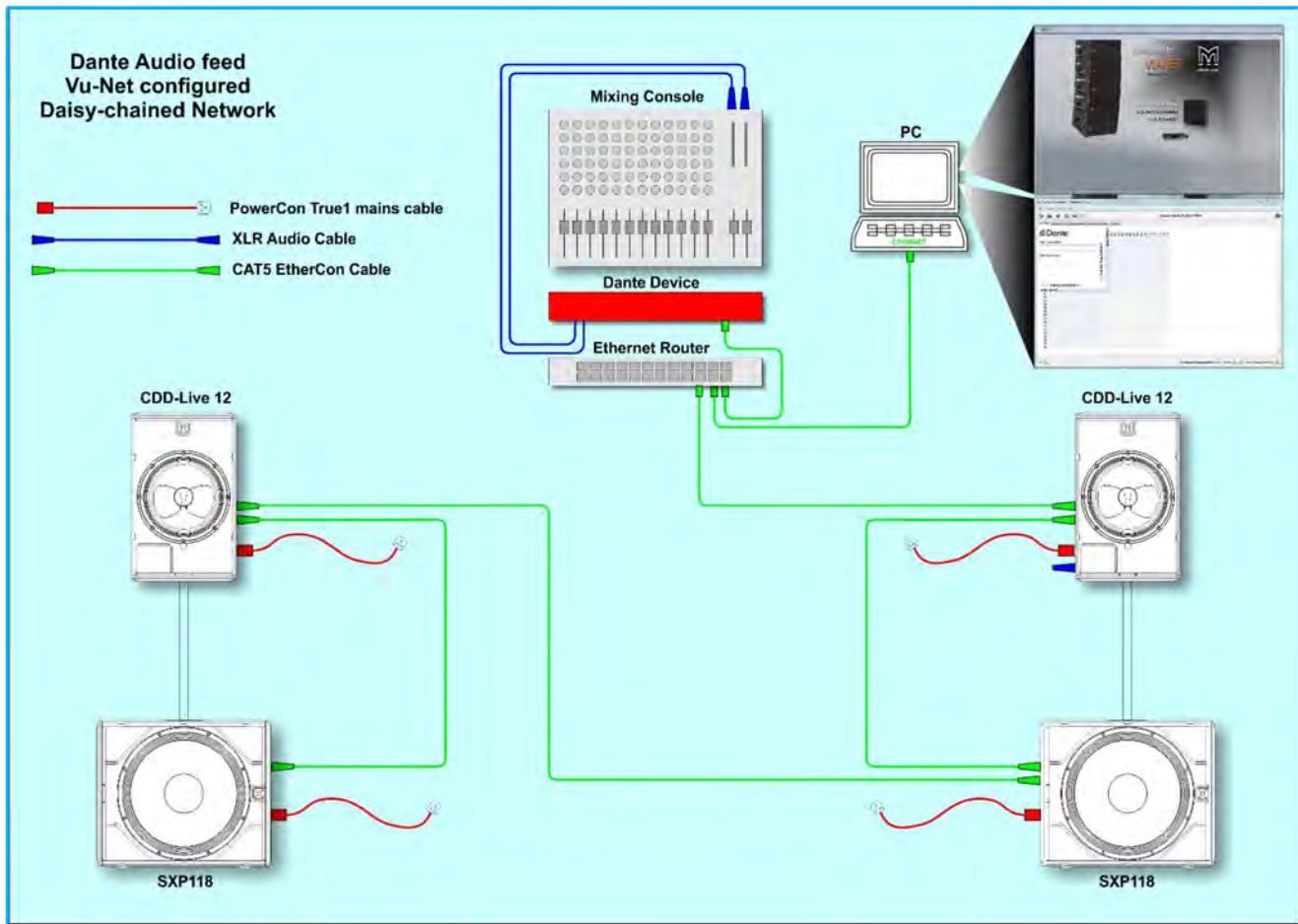
This system demonstrates the simplest implementation of Dante. The analogue audio connections to each cabinet are no longer required, a Dante feed is derived from your audio source using one of the hundreds of Dante enabled devices. The diagram shows an analogue mixing console routed to a Dante interface such as a DX4.0 or one of the Focusrite RedNet range however this could be a digital mixing console, a great many of which have Dante outputs either as standard or as an option.
