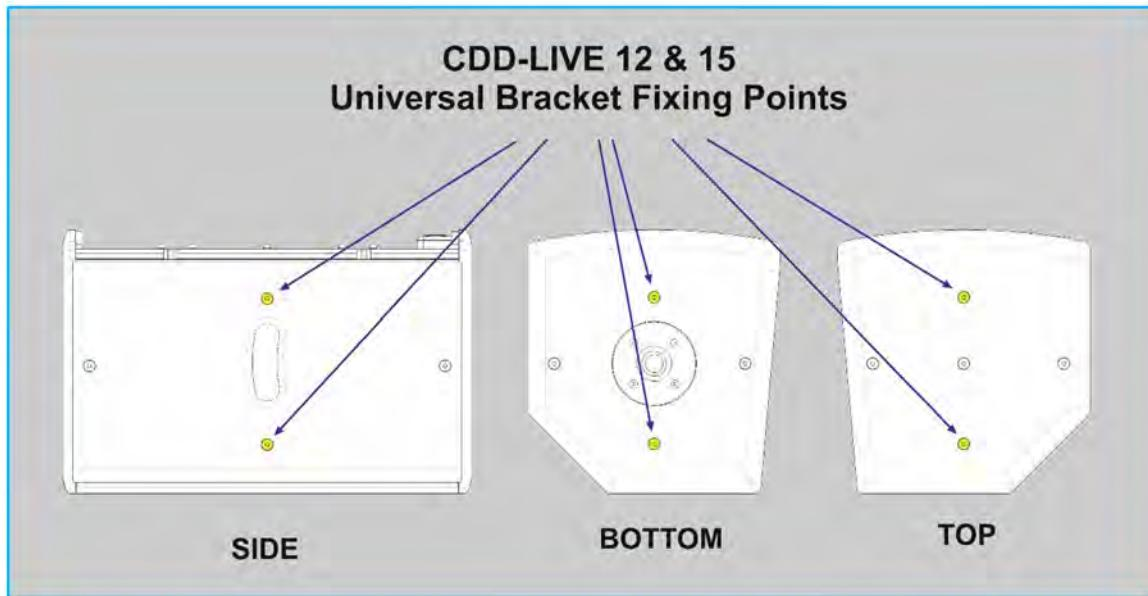
The screws that you have removed are no longer required, the bracket MUST be attached with the M8 x 35mm screws supplied with the Universal Bracket. The screws that are supplied in the cabinet are not long enough and not rated for suspending the cabinet so will be unsafe.
