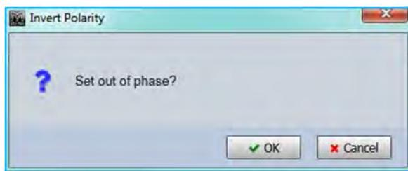
On clicking 'OK' the phase will be inverted and the Polarity button will turn green; -
