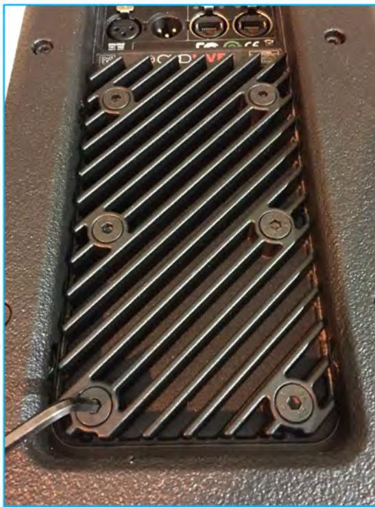
Position the bracket over the required holes orientated to suit the orientation that is being used and screw into place tightly using the bolts supplied with the bracket (note that you cannot use the bolts removed from the heatsink as they are too short).
