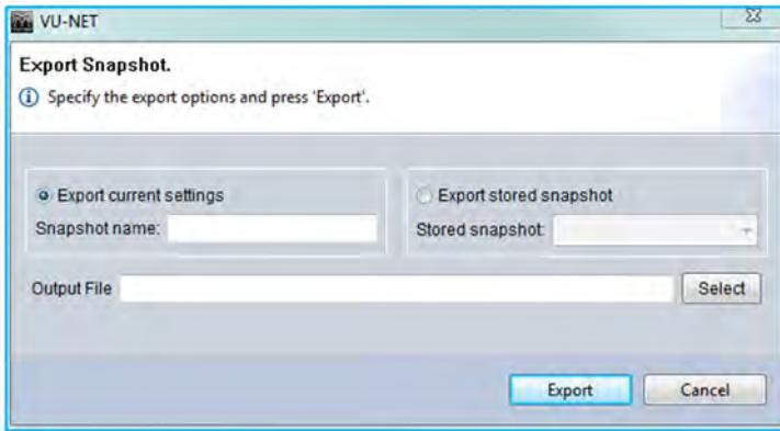
You can choose to select the current active settings, a true snapshot of the system configuration, or to export one of the four Snapshots stored in the cabinet DSP. If you choose to Export the current settings, you should first give the Snapshot a name so it is easy to identify when it is imported back into a cabinet "CDD-Live8 Stereophonics" for example.
