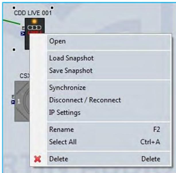
'Open' has exactly the same function as double clicking on the speaker icon to open the full control window.
