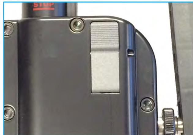
Once at the desired height the handwheel is tightened to secure the pole in position and the crank handle can be folded away
