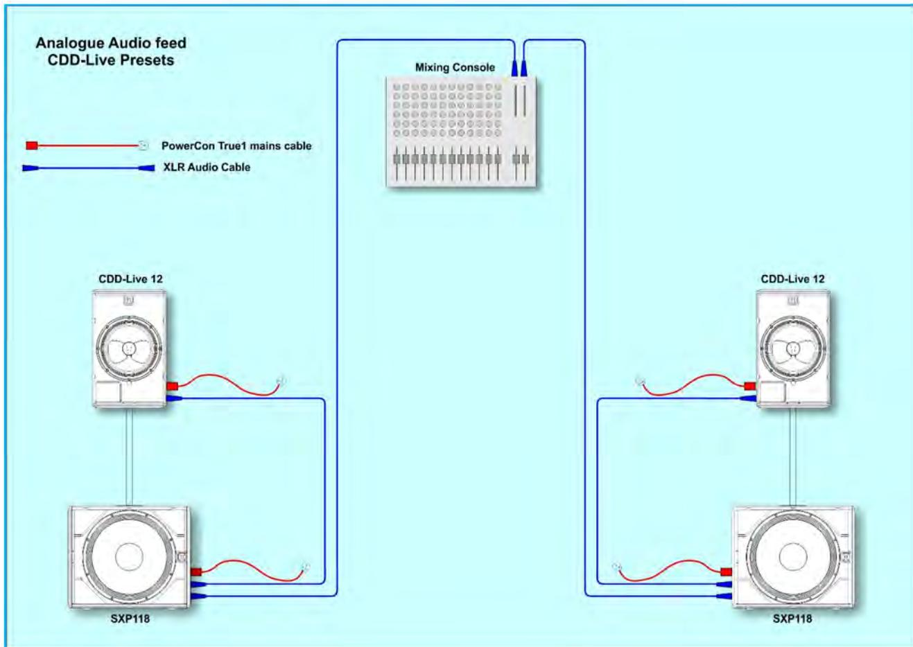
This illustrates the simplest deployment of a stereo CDD-Live system. Analogue Audio from your source is routed to left and right, it is connected to the SXP118 subs, the parallel out is used to link up to the CDD-Live 12s. In this example Preset 1 would be selected on the SXP118 and Preset 2 on the CDD-Live 12s. All crossover and equalisation processing is taken care of by the internal DSP using the selected presets.
