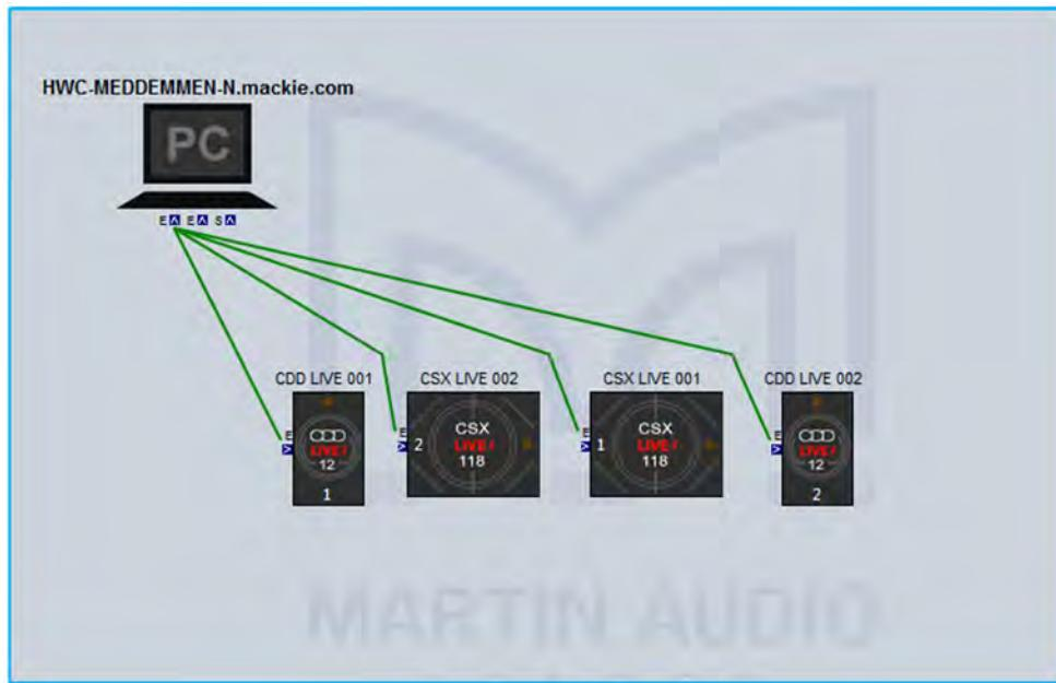
Each CDD-Live device will be shown as an icon which includes the front grille LED. If you click on the cabinet to select it you can then click on the LED which will illuminate on the icon and on the speaker to make it easy to identify which cabinets you are controlling, useful particularly when you are arranging the overview screen in Vu-Net to represent the physical positioning of the system;-
