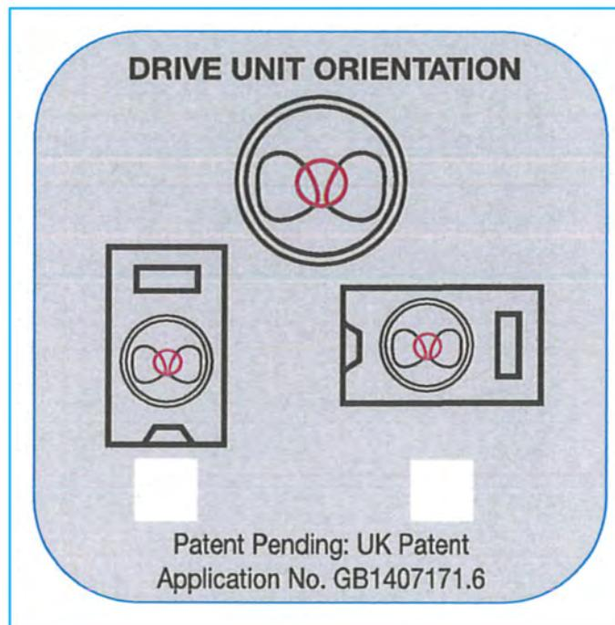
Re-fit all driver mounting screws tightly, rotate the badge as mentioned above and replace the grille as previously described.
