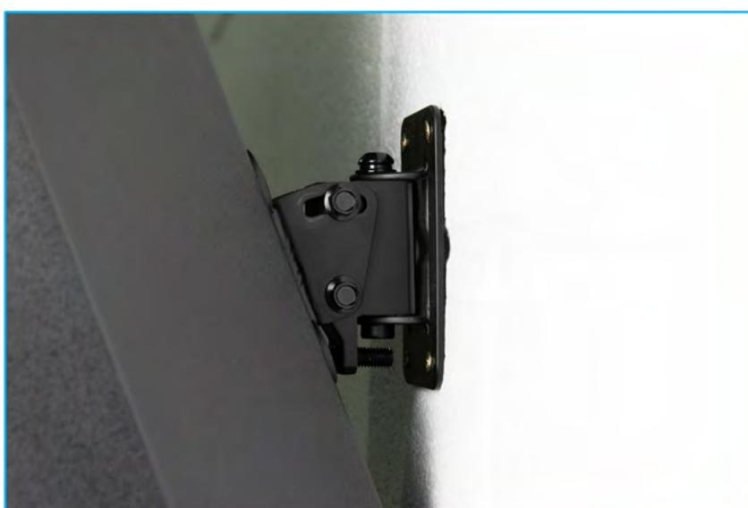
Final adjustments can now be made. Horizontal (pan) adjustment is available by rotating assembly on the vertical bolt, when you're happy with the angle, the vertical securing bolt can be tightened with an M5 hex key (CDDWB8/6) or an M6 hex key (CDDWB10/12) to lock the position.
