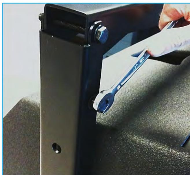
Note that for portable use it is advisable to fit the scaffold clamp or pole mount adaptor before attaching the yoke to the cabinet. For fixed installations the yoke would be attached to the wall or ceiling using appropriate fixings and then the cabinet fitted to the yoke.
