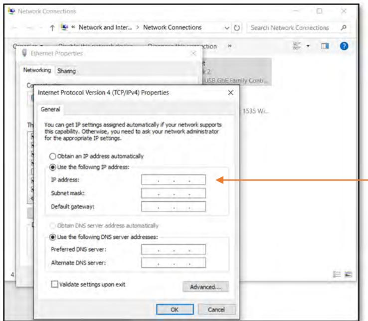
Check 'Use the following IP address' and type in an IP address within the range of your unit. Make sure this IP address is not in use (should not appear on your ARP table above). You can use any IP address that is not in that table, but you must ensure it is within the same range as your unit.
