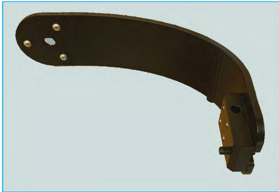
Second stage is to fit the cabinet bracket in place. The bracket is attached orientated as shown by removing four screws in the rear heatsink with an M4 hex key and attaching the bracket with the same screws. The 4 screws in the middle of the cabinet must be used to allow fitting in landscape.
