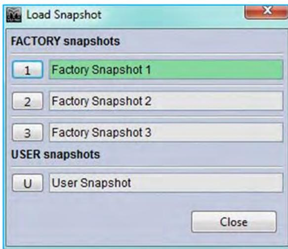
'Save Snapshot' is the function used to store parameters that you have edited to the User Location "U". This location can be recalled using the Load Snapshot command or by selecting Snapshot 4 using the button on the speaker connector panel. To store a Snapshot once you have made all the parameter changes that you need, select 'Save Snapshot', you will see this window;-
