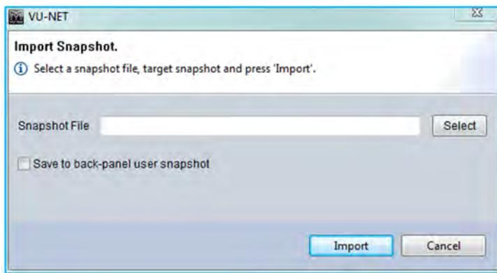
Click on the 'Select' button to navigate to the location on your PC where your CDD-Live files are located. If you would like to store the imported snapshot directly to the User Snapshot location so it can be stored and selected in future without a PC connected click on the 'Save to back-panel user snapshot' box. If this is left un-checked the snapshot settings will be imported but will be lost when a new snapshot is selected from the rear panel switch.
