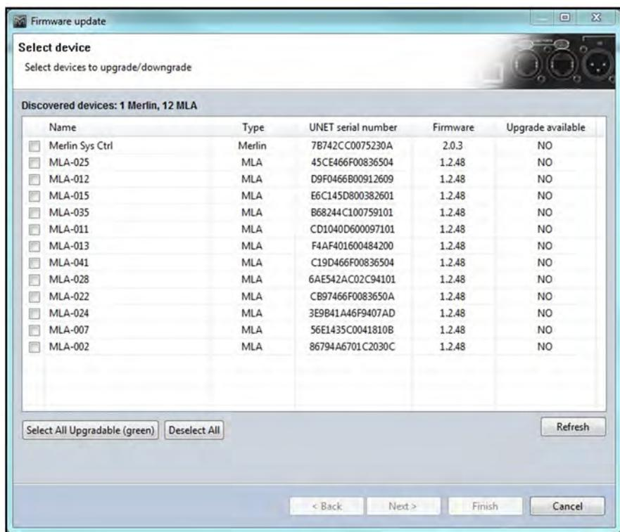
Vu-Net compares the discovered Firmware version with the latest version stored in its database and will indicate in the final column whether an upgrade is available. In this instance a single Merlin and twelve MLA have been found and all have up to date firmware however we can still proceed with an update to show how the process works.
