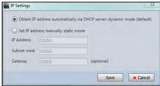
If you select Static IP you will need to enter a manual IP address and subnet mask in the same range as all other devices on the network that you need to communicate with. If you click on 'Set IP address manually: static mode', the IP address, Subnet mask and Gateway windows previously greyed-out will become available; -
