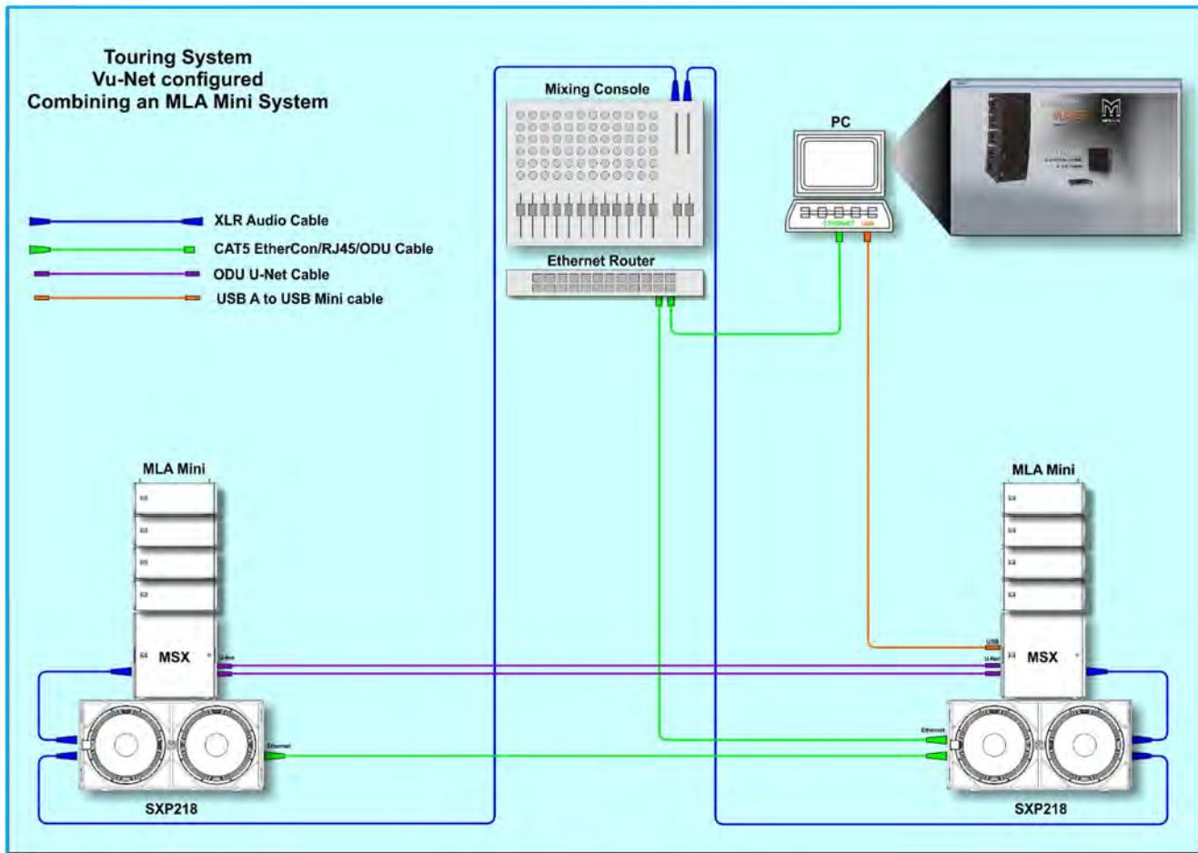
As mentioned in option 6, CDD-Live and SXP speakers can easily be integrated with MLA Mini systems. A practical example might be to use a pair of SXP218 subwoofers to extend the low frequency response of an MLA Mini system in larger venues. The MLA Mini system is set up in the usual manner with a USB connection from the PC to the first MSX and a pair of U-Net cables link the two MSX creating a closed loop to provide redundancy.
