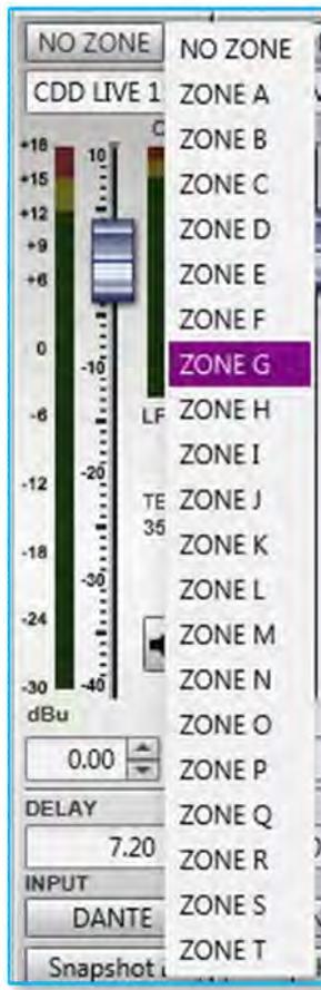
Click on the desired zone and it will be displayed on the zone button. The zones are colour coded to make it instantly obvious which cabinets are on the same zones. Colours are as follows; -
