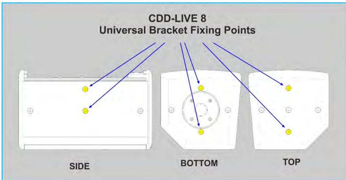
Position the universal Bracket and screw in place using the screws removed from the cabinet, ensure that they are fully tightened. If fitting to the side of the cabinet note that you attach through the central hole in the bracket and the one at the back, fitting to the top and bottom the holes at the front and back are used, the central hole is not used.
