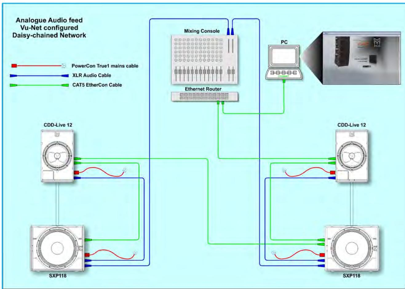
With this system the audio feed remains exactly as with the basic system sending a stereo analogue audio feed to the cabinets. Control over the system has been enhanced by adding a network.
