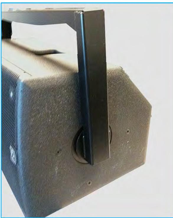
Then attach the upper arm to the top of the cabinet through the central M8 insert from which the M8 screw was removed. Use either the M8 handwheel or the M8 x 40mm bolt. Use the spring washer (first) then the plain washer (second) onto whichever fixing you are using, pass it through the hole in the mounting plate and into the cabinet insert. Tighten it sufficiently to make handling easy but allow for final adjustment.
