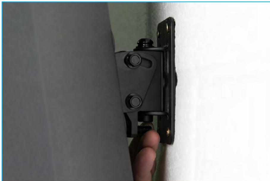
Once the vertical position is fixed the two horizontal bolts can be tightened, this is best achieved by using a socket set with an extender bar to reach the bolt heads.
