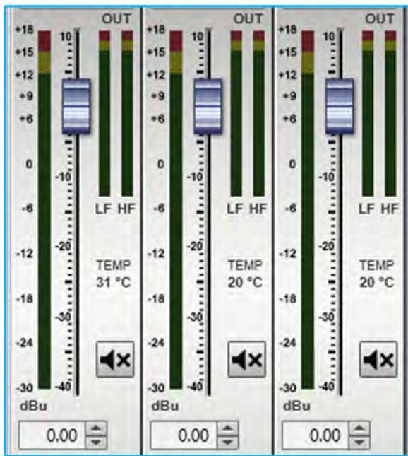
There is also a temperature read out showing the temperature of the DSP and amplifier module; -
