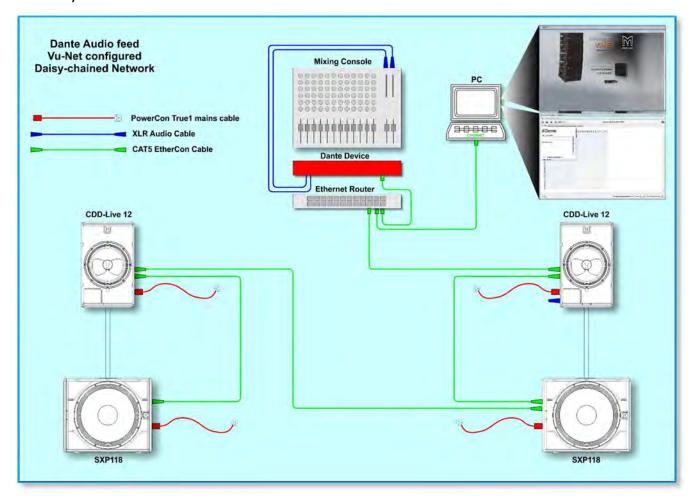
This system demonstrates the simplest implementation of Dante. The analogue audio connections to each cabinet are no longer required, a Dante feed is derived from your audio source using one of the hundreds of Dante enabled devices. The diagram shows an analogue mixing console routed to a Dante interface such as a DX4.0 or one of the Focusrite RedNet range however this could be a digital mixing console, a great many of which have Dante outputs either as standard or as an option.
