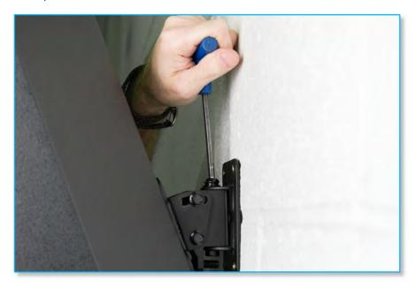
Vertical (tilt) adjustment is made by adjusting the grub screw:
