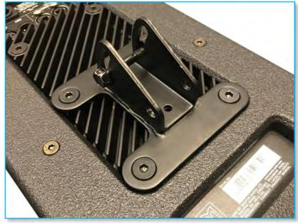
You are now ready to fit the speaker to the wall. Offer the speaker up to the bracket so you can hook horizontal bolt in the curved slot onto the notch on the ball bracket. Make sure that you follow appropriate safety measures if you are working at height such as using a scaffold tower or lifting platform which allows you to safely use both hands for this.
