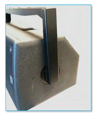
Then attach the upper arm to the top of the cabinet through the central M8 insert from which the M8 screw was removed. Use wither the M8 handwheel or the M8 x 40mm bolt. Use the spring washer (first) then the plain washer (second) onto whichever fixing you are using, pass it through the hole in the mounting plate and into the cabinet insert. Tighten it sufficiently to make handling easy but allow for final adjustment.
