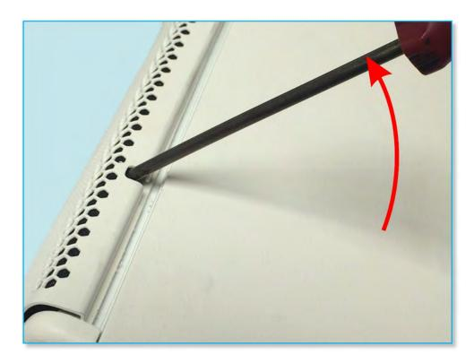
Repeat this process for the remaining gaps in the grille to ease it out of the slot all the way up one side of the cabinet; when you get to the final gap the grill should pop out and away from the front of the cabinet.
