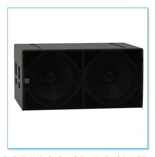
The SXP218 achieves the ultimate in subwoofer performance for the most demanding professional applications – delivering very high output levels and superb transient performance with minimal distortion. With an operating range of 35Hz- 150Hz  $\pm$  3dB, it houses dual 18'' long-excursion (460mm)/4'' (100mm) voice coil drivers with water-resistant cones and triple roll surrounds.
