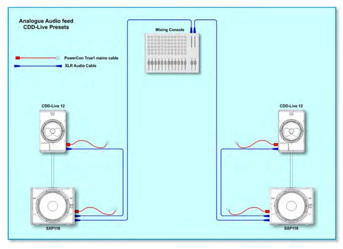
This illustrates the simplest deployment of a stereo CDD-Live system. Analogue Audio from your source is routed to left and right, it is connected to the SXP118 subs, the parallel out is used to link up to the CDD-Live 12s. In this example Preset 1 would be selected on the SXP118 and Preset 2 on the CDD-Live 12. All crossover and equalisation processing is taken care of by the internal DSP using the selected presets.
