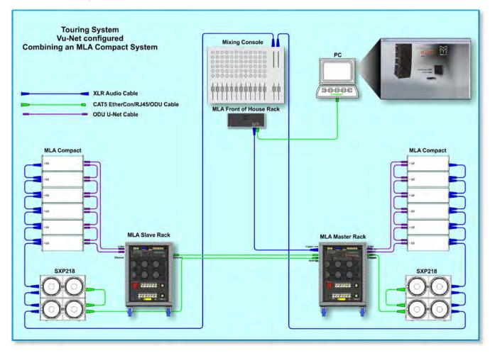
In this example the SXP218 subs have been deployed with an MLA Compact system as a lower cost alternative to the DSX or MLX subwoofer. Much of the infrastructure is based around the standard MLA compact system components.
