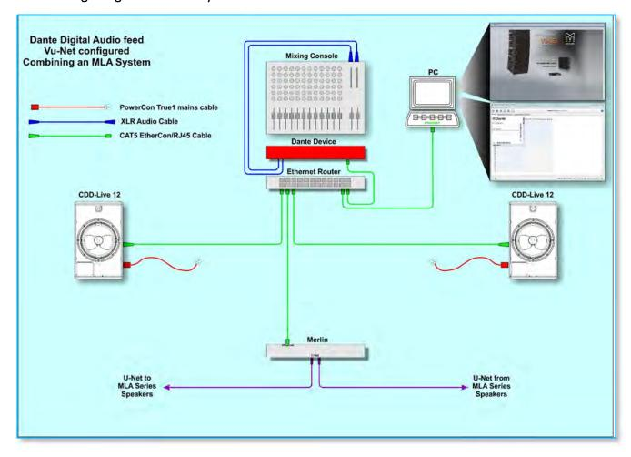
CDD-Live is ideally suited to being integrated with a Martin Audio Multicellular system, the entire system can be managed via a single Vu-Net project.
