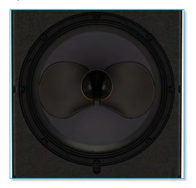
Be careful not to push the screwdriver in to far which could easily damage the cone suspension. Lever the driver up enough to get your fingers under the edges of the driver. Lift it up just enough to get a firm grip, do not put any strain on the connecting wired. Rotate the driver through 90° either clockwise or anticlockwise depending on your application. Check that the driver is at the correct orientations as shown below; -
