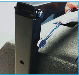
Note that for portable use it is advisable to fit the scaffold clamp or pole mount adaptor before attaching the yoke to the cabinet. For fixed installations the yoke would be attached to the wall or ceiling using appropriate fixings and then the cabinet fitted to the yoke.
