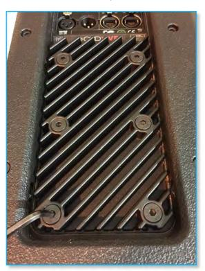
Position the bracket over the required holes orientated to suit the orientation that is being used and screw into place tightly using the bolts supplied with the bracket (note that you cannot use the bolts removed from the heatsink as they are too short).
