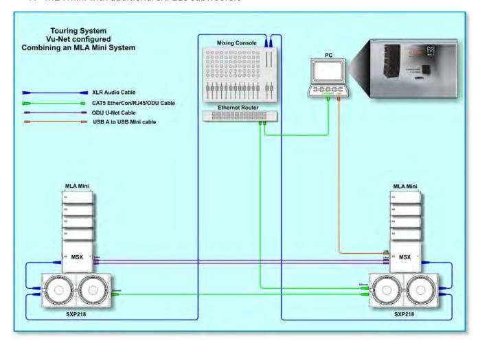
As mentioned in option 6, CDD-Live and SXP speakers can easily be integrated with MLA Mini systems. A practical example might be to use a pair of SXP218 subwoofers to extend the low frequency response of an MLA Mini system in larger venues. The MLA Mini system is set up in the usual manner with a USB connection from the PC to the first MSX and a pair of U-Net cables link the two MSX creating a closed loop to provide redundancy.
