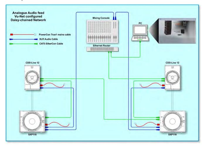
With this system the audio feed remains exactly as with the basic system sending a stereo analogue audio feed to the cabinets. Control over the system has been enhanced by adding a network.
