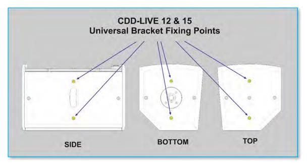
The screws that you have removed are no longer required, the bracket MUST be attached with the M8 x 35mm screws supplied with the Universal Bracket. The screws that are supplied in the cabinet are not long enough and not rated for suspending the cabinet so will be unsafe.
