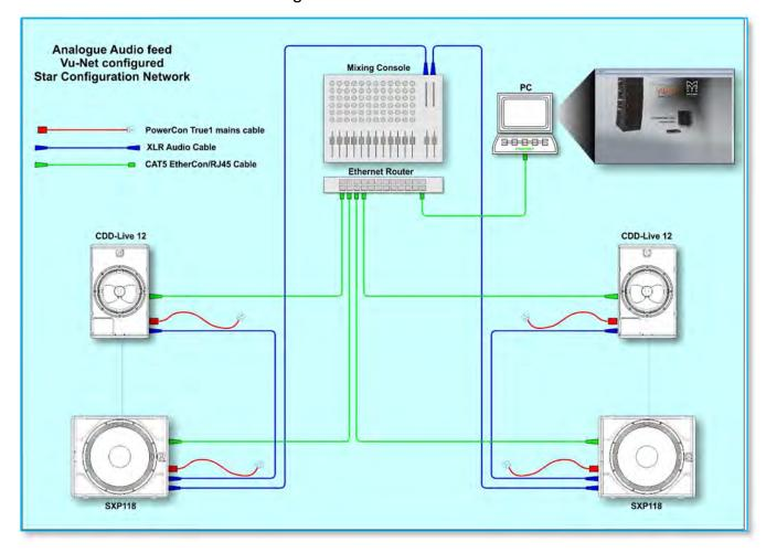
As with our example number two, analogue audio is routed to our left and right speakers and we can control the parameters in depth using Vu-Net, in this example however, the network connection to each cabinet is made with an individual Ethernet cable from an Ethernet router (note that the router must include a DHCP server unless the entire system is configured for Static IP).
