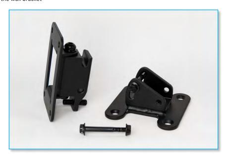
First fix is to secure the wall section of the bracket. This is the part with four mounting holes, a vertical bolt holding the section which allows horizontal adjustment and the slot into which the cabinet bracket bolt sits. Use appropriate wall fixings suitable for the composition of the wall. These must be of sufficient strength to support the weight of the speaker, 14Kg for the CDD-Live 8 and 28Kg for the CDD-Live 12.
