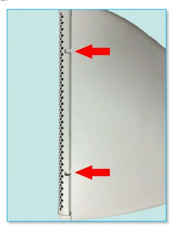
Insert the screwdriver blade into one of the gaps - either at the top or bottom of the cabinet (don't start in the middle).
