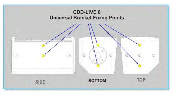
Position the universal Bracket and screw in place using the screws removed from the cabinet, ensure that they are fully tightened. If fitting to the side of the cabinet note that you attach through the central hole in the bracket and the one at the back, fitting to the top and bottom the holes at the front and back are used, the central hole is not used.
