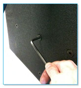
To fit the yoke first the upper arm needs to be pivoted upwards so there is enough room to locate the spigot into the speaker top hat. The upper arm is attached with two M8 bolts, the bolt in the corner acts as a pivot and the second bolts approximately 60mm along the upper arm from the corner locks the arm in place to prevent it from pivoting so this screw needs to be temporarily removed using the 13mm spanner;-
