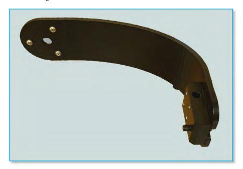
Second stage is to fit the cabinet bracket in place. The bracket is attached orientated as shown by removing four screws in the rear heatsink with an M4 hex key and attaching the bracket with the same screws. The 4 screws in the middle of the cabinet must be used to allow fitting in landscape.
