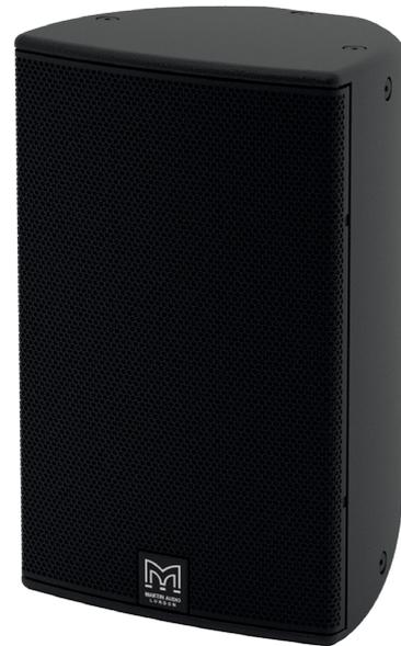
The CDD10 is a very compact two-way passive loudspeaker system which utilises a 10" (250mm) LF/1" (25mm) exit HF Coaxial Differential Dispersion driver. It is uniquely placed to meet the foreground requirements of music bars and clubs, as well as the varied architectural applications that require upfront sound levels from a very compact enclosure. Use with a CSX118 or CSX218 subwoofer will enable the CDD10 to operate as small dancefloor system that is remarkably powerful for its size.
