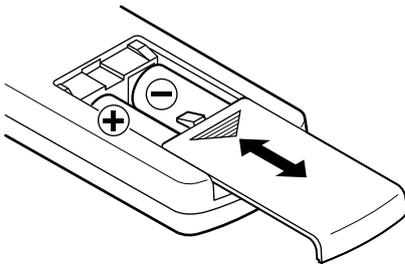
2. Confirm +/- polarity, and insert two AA batteries.
