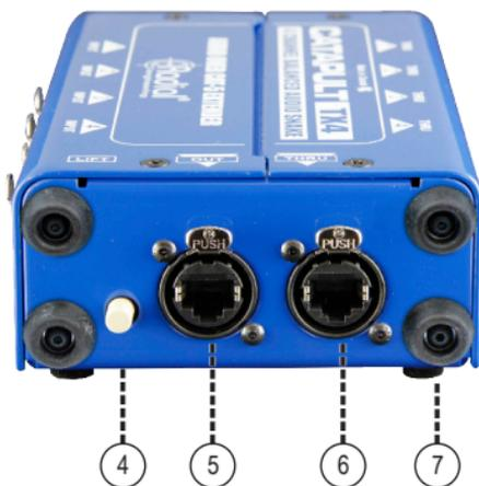
4. **LIFT:** Lifts the Cat 5 cable ground path to help eliminate troublesome ground loop noise.
