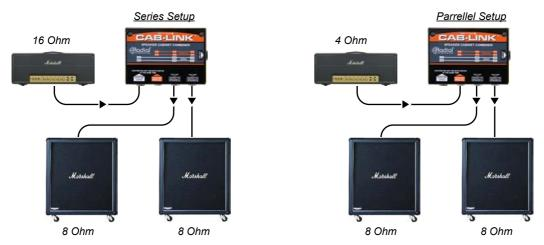
Ensure that both cabinets have the same impedance in Ohms ( $\Omega$ ).
