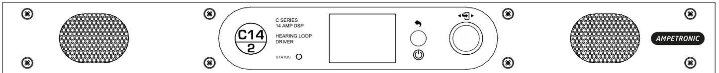
Depending on a number of factors regarding the installation of the loop and the set-up of the driver, the C Series can provide compliance with IEC 60118-4 for perimeter loop areas of up to 950m<sup>2</sup> or phased array systems up to 3,200m<sup>2</sup>.
