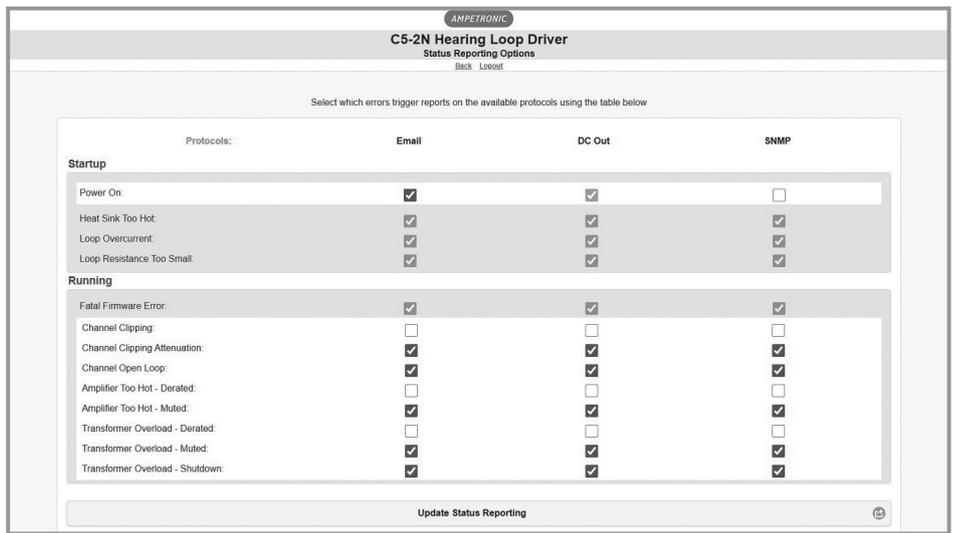
On C10/14 drivers the middle column sets the conditions which activate the both the status relay and the DC Out.
