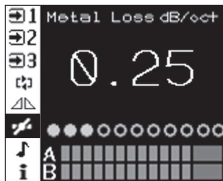
Metal Loss Correction value adjusted by rotary control. In 0.25dB steps from Off (0dB) to 4dB/Octave. Clockwise from 4dB/Octave sets MLC to 'Custom' – this is only configurable via the network connection (where fitted)
