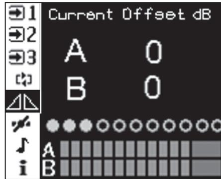
Current Offset value adjusted by rotary control. Counter clock-wise reduces channel A. Clock-wise reduces channel B. Adjustment is from 0 to -10dB on either channel. Further adjustment turns that channel off and disables loop test for that channel.
