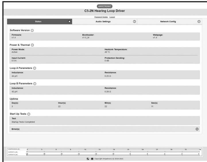
**Software Version:** The version of the bootloader, the firmware in the driver and the version of the website. In order to update firmware, please refer to Section 13.
