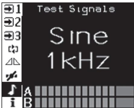
Loop Current bar graph for each channel. Shows Loop output current in 2dB steps from >-20dB to 0dB in green. Red = clipping
