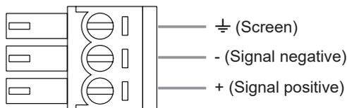
**Microphones:** Suitable dynamic or condenser microphone with balanced cable feed. Select phantom power as required. Connect to INPUT 1 and INPUT 2 (with selector switches in the appropriate position) using a 3-pole plug wired as per Connections drawing.
