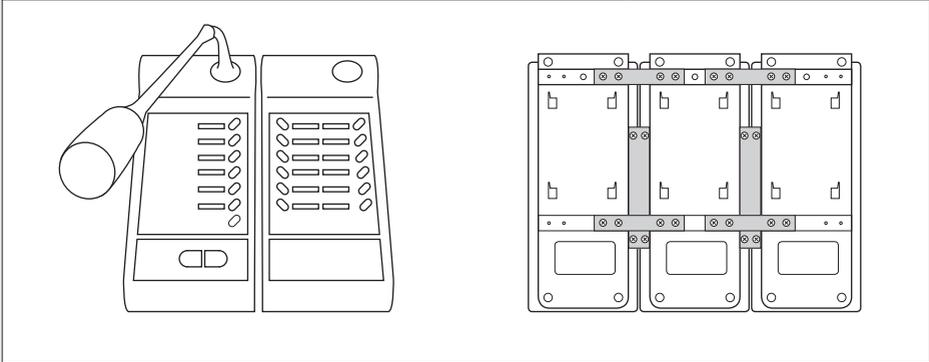
Connect all BM 2006 paging microphones (daisy-chained through CAT5 cable), as according to the following figure:
