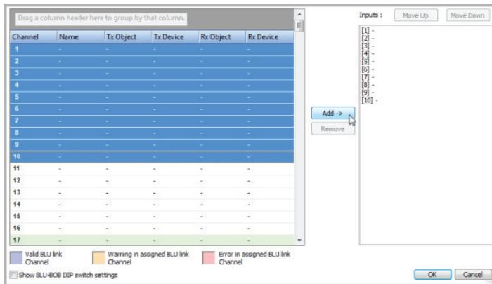
Click OK to accept and close the window. The BLU Link Input object is now configured and ready to be wired to other objects. Wiring to an Audio Coupler object allows signal names to be added to the incoming BLU Link channels.
