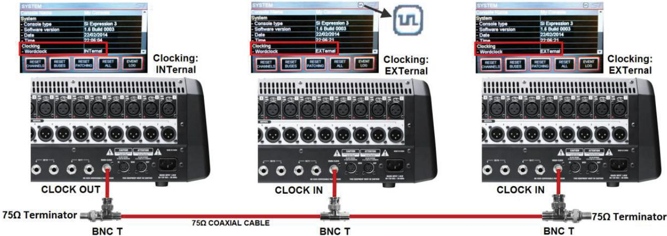
2. Use an external generator to distribute word clock to each console. Set BLU-SI option card as instructed above. All consoles will be deriving their word clock from an external source. These must have the Wordclock set to EXTernal.
