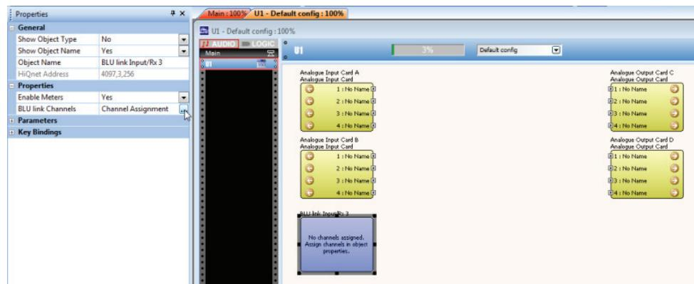
In the Channel Assignment window select the desired channels in the list in the left-hand list then click Add. (Use the SHIFT key to select multiple consecutive channels or use the CTRL key to select multiple non-adjacent channels)
