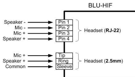
**Caution: Do not connect to both jacks simultaneously.** Doing so risks damaging the connected devices. Before connecting to either jack, ensure that the internal jumper is set to the appropriate position. By default, the BLU-HIF ships with the jumper in the Headset **RJ-22** jack position. For more information on setting the internal jumper, please refer to the BLU-HIF Installation Guide.
