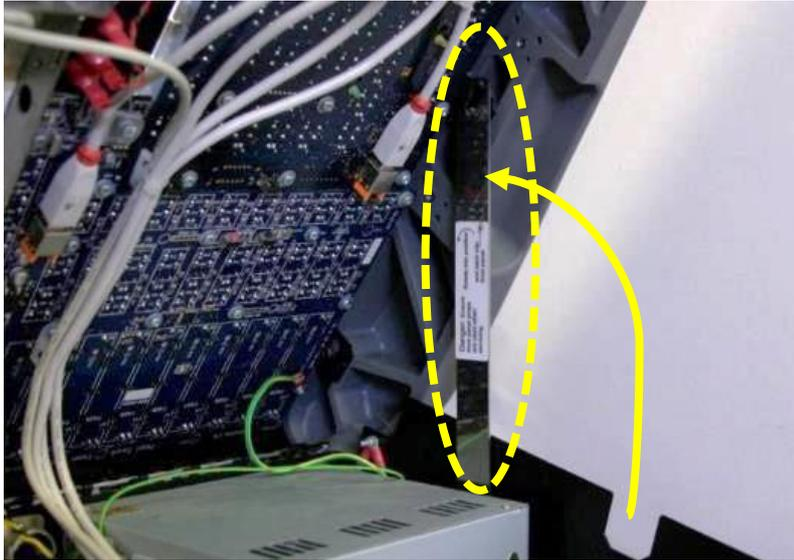
A. Cut the cable-tie and disconnect the Touch Sensor USB cable
