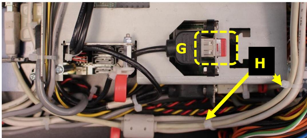
H. Close the console, stow the stand correctly so it can not touch the UPS.
