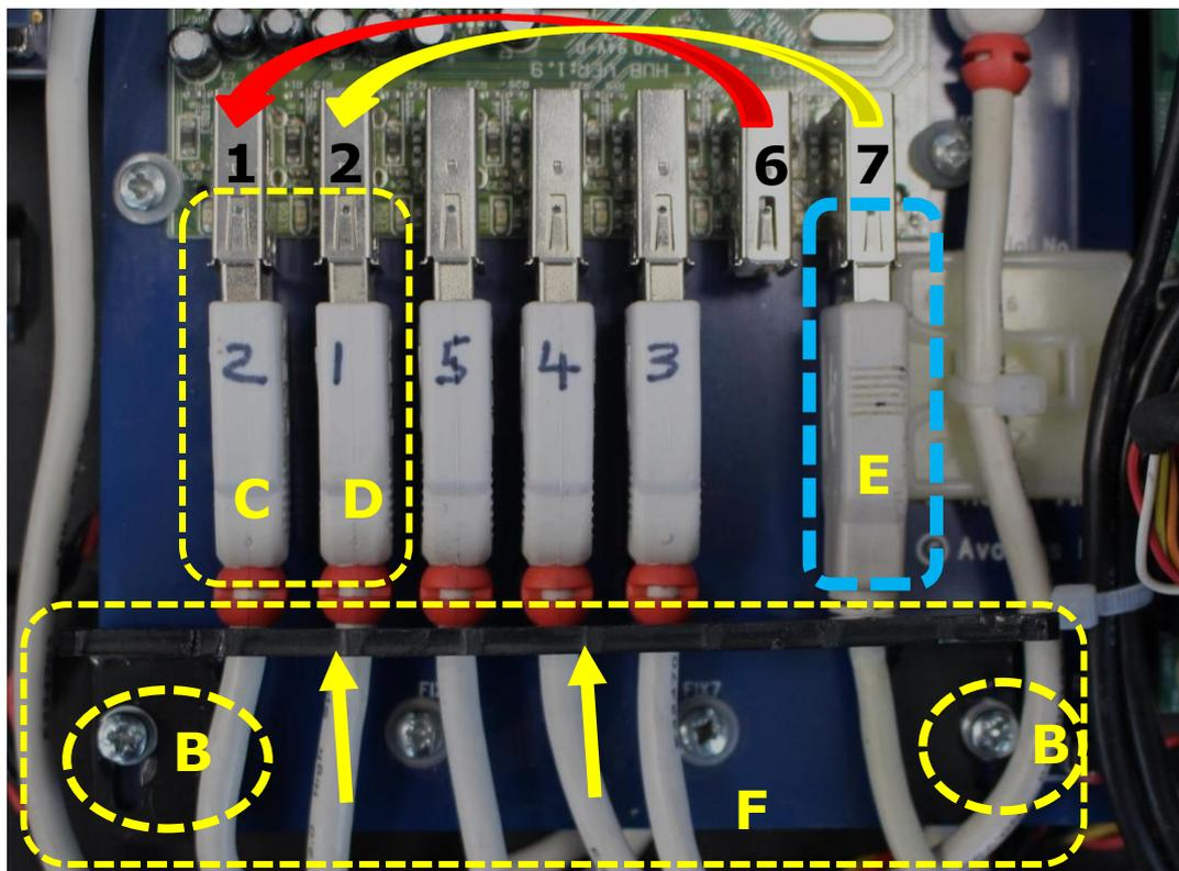
F. Plug the AvoKey into the USB port on top of the safety frame.
