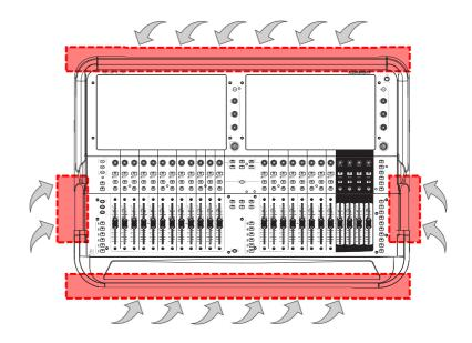
Leave adequate space for ventilation (\*) at the sides of the mixer in the area indicated.
