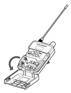
Insert the batteries according to the plus (+) and minus (-) marks found inside the battery compartment.
