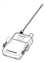
2 Open the battery cover while holding the latches down.
