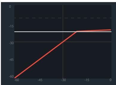
When the limiter threshold is lower than the compressor threshold, the compressor threshold is cleared, and only the limiter threshold is displayed.
