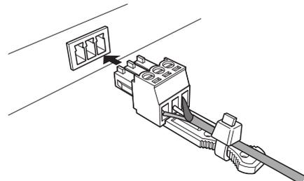
3. Verify the pin assignments, and connect each to the applicable wire.
