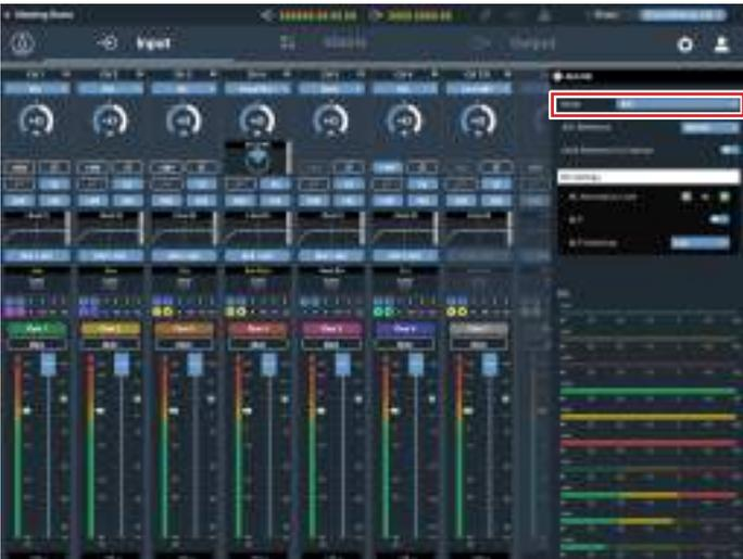
3. From "AEC Reference", select the reference signal (the signal for removing echoes).
