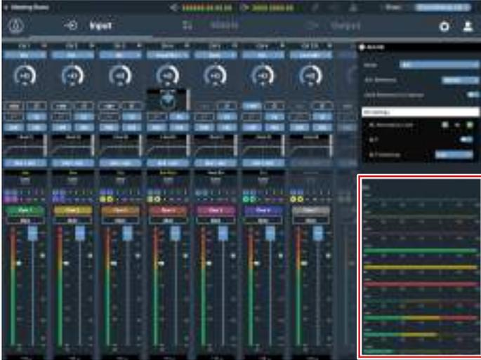
7. Until the ERL meter is at 0 or less, adjust the distance between microphones, speaker positions, input level, etc.
