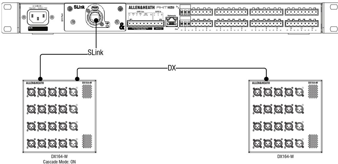
A DX Hub can be connected to the SLink card for further expansion with up to 8 DX expanders. It also enables a single cable link to the AHM processor in cases where multiple expanders are located on a different floor, area or building.
