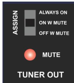
*You can also use the TUNER OUT as an output to an amp. Select OFF W MUTE when switching instruments.*
