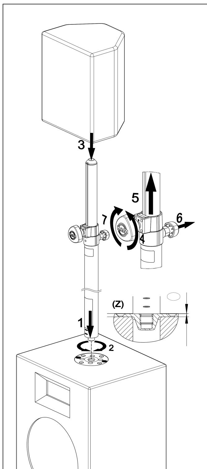
The locking screw must be screwed into the clamp once before first use.
