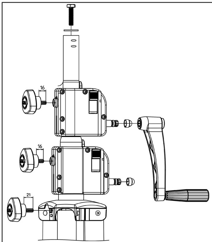
The clamping screws must be screwed into the crankcase and the base clamp once before first use.
