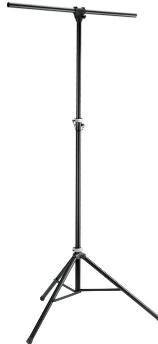
Lightweight aluminum lighting stand with cross bar. Stable folding 3-leg construction. Height and feet adjust by an easy-to-use clamping lever. Additional safety pin ensures secure support. Cross bar with boreholes for up to 8 spotlights. Optional corresponding screw fitting set 24621 available.
