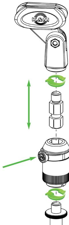
To remove the threaded bolt or to change the equipment, press the K&M logo on the grey locking ring and remove the threaded bolt upwards from the Quick-Release Adapter.
