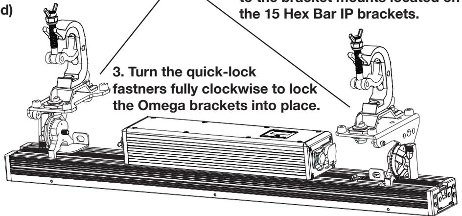
3. Turn the quick-lock fasteners fully clockwise to lock the Omega brackets into place.
