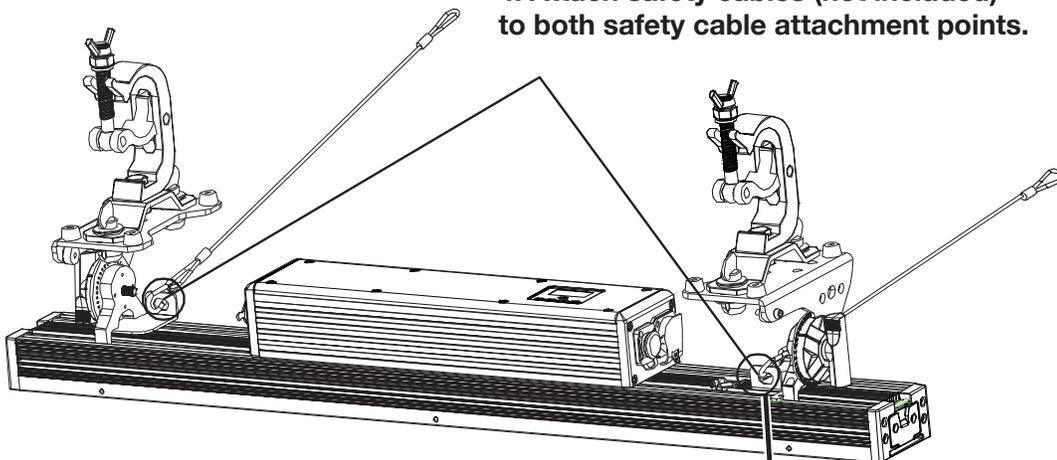
4. Attach safety cables (not included) to both safety cable attachment points.
