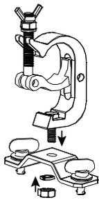
1. Attach a clamp (not included) to each omega bracket.
