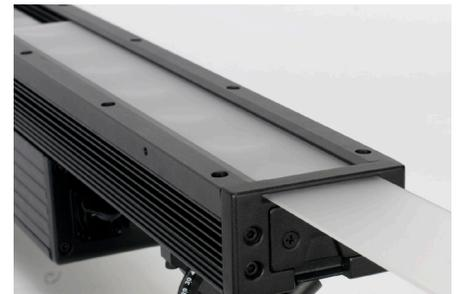
Locate the filter slot door located at either end of the unit. Pull and hold the slot door down and gently slide the frost/diffuser filter in. Make sure the filter is all the way inside before releasing the slot door to close.
